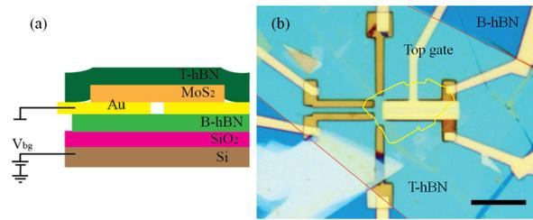
FIG. 1. (a) Schematic and (b) optical microscopy of the bottom contact Au/MoS<sub>2</sub>. Outline shows the edge of monolayer flake. The scale bar is 10  $\mu\text{m}$ .
