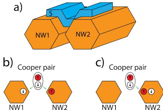
FIG. 1. (a) Schematic of a double NW device with an S island. The red asterisks indicate the formation of parafermions. (b) and (c) Illustrations of pairing by CPS and LAR, respectively.
