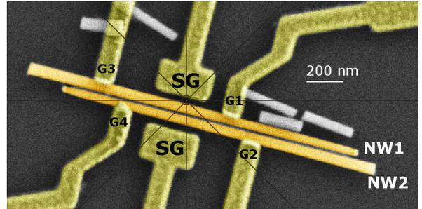
FIG. 2. False-color SEM image of a parallel NW device. Two InAs nanowires (NW1 and NW2) with  $\sim 40$  nm diameter are individually contacted by normal metal gold contacts (G1-G4) and tuned capacitively by two sidegates (SGs).
